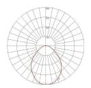
ODV 18W 4000K (1,327.8lm (Lamp), 566.3cd (Max intensity), 17W (Power))
