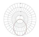
ODV 12W 4000K (963lm (Lamp), 400.8cd (Max intensity), 11W (Power))
