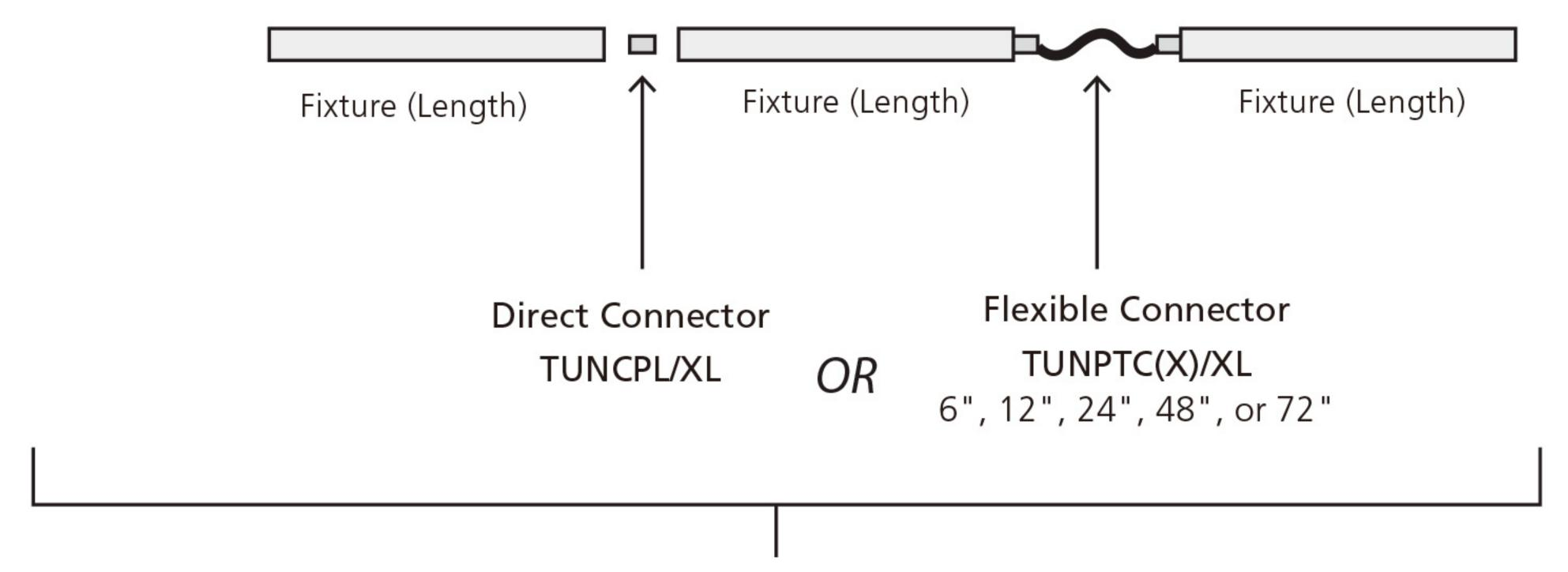
400 WATT MAX LOAD PER POWER CORD OR HARDWIRE BOX(NON-DIMMING)
